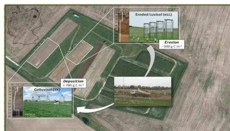
The CarboZALF-D approach: combining topsoil translocation and CO_2 flux measurements by automatic chambers
